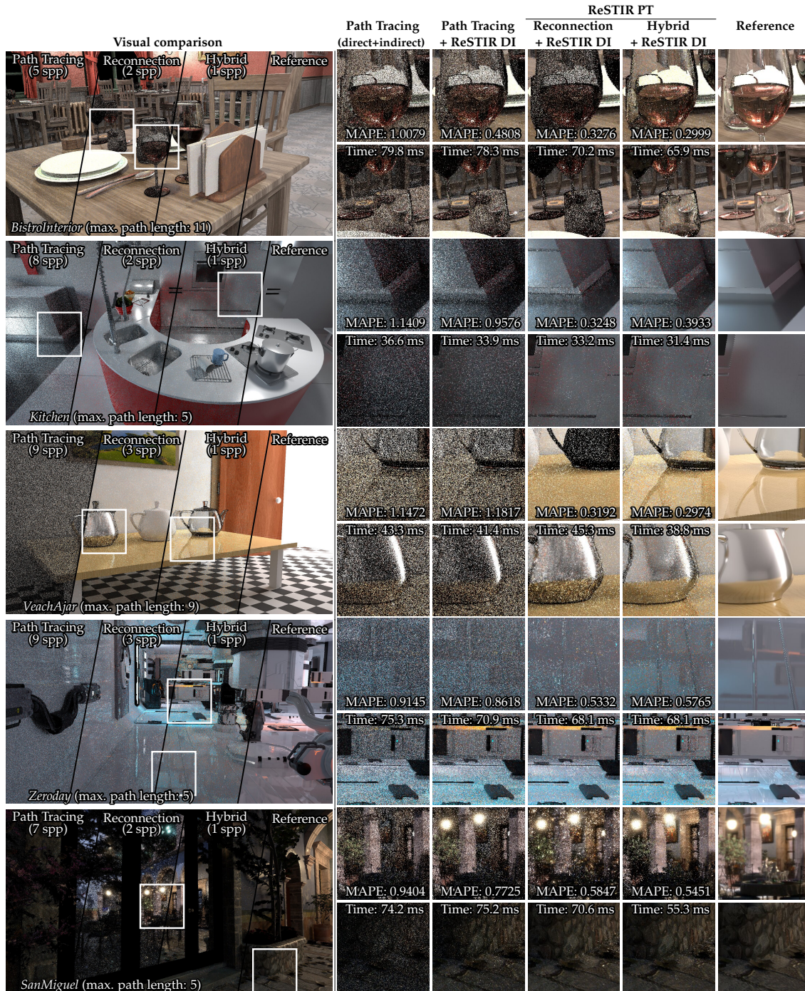
Figure 6.13: Comparing path tracing and two variants of our ReSTIR PT (reconnection and hybrid shift) for real-time rendering (all methods use ReSTIR DI for direct light). Images are captured during an animation sequence. MAPE are computed using HDR images.
