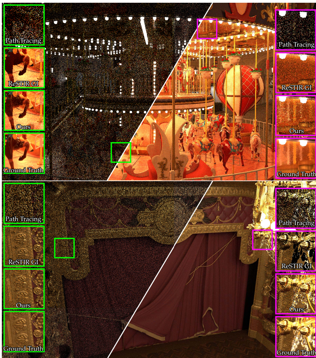
Figure 6.1: Our new generalized resampled importance sampling (GRIS) theory extends resampled importance sampling [8] to guarantee convergence even when applied to correlated samples arising from spatiotemporal reuse (i.e., Bitterli et al. [7]). GRIS allows applying ReSTIR to reuse arbitrary paths, shown with paths of length 10 in the Carousel (top) and Paris Opera House (bottom). Main images compare naive path tracing and our new ReSTIR PT in equal time (80 ms at 1920 \times 1080 ). Insets show equal-time path tracing, ReSTIR GI [10], our ReSTIR PT, plus a converged reference. We significantly improve quality for glossy interreflection, reflections, refractions, and other high-frequency lighting. For Carousel , MAPE errors: path tracing (1.63), ReSTIR GI (0.45), and ReSTIR PT (0.39). Corresponding errors in Opera House : 1.28, 0.39, and 0.33. ( Carousel ©carousel_world; Paris Opera House courtesy ©GoldSmooth from TurboSquid.)
