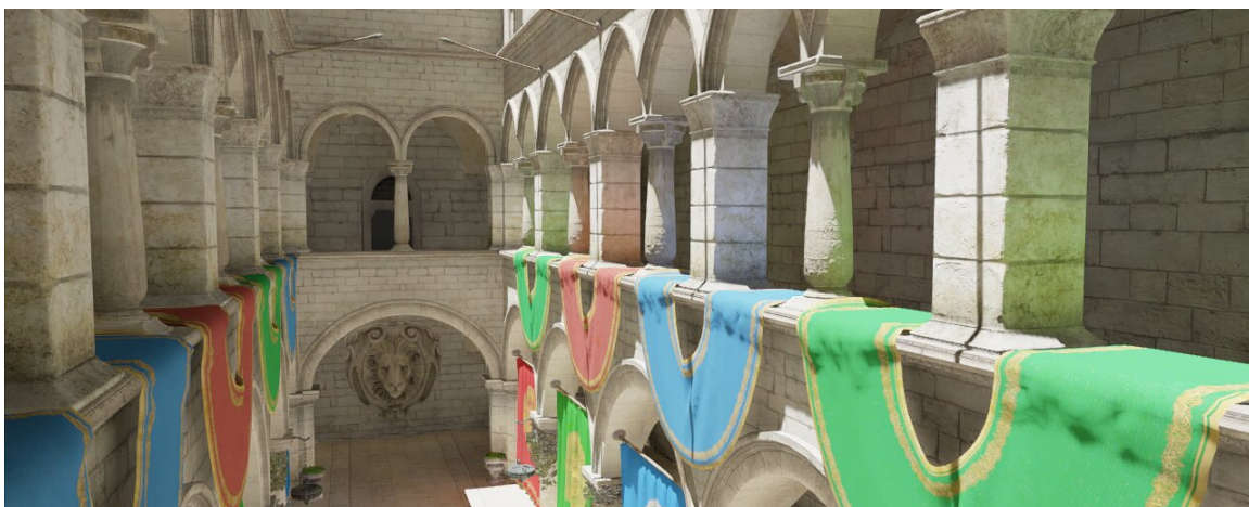
Figure 3.1: An example frame rendered using our real-time global illumination solution with one million virtual point lights, computed by our method, using \alpha = 2 and 4 \times 4 interleaved sampling. The render time is 24 ms on an NVIDIA RTX 2080 GPU at 1280 \times 720 resolution.
